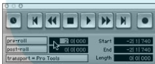
Figure 4-4: Clicking the Pre-Roll or Post-Roll field lets you enter a value for the pre/post roll.
